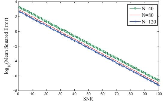
**Fig. 2.** Logarithm of the mean squared error of the recovered signal compared to the original signal
