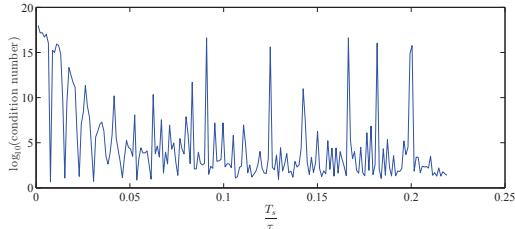
**Fig. 3.** Logarithm of the condition number of the linear system for the ratio  $\frac{T_s}{\tau}$
