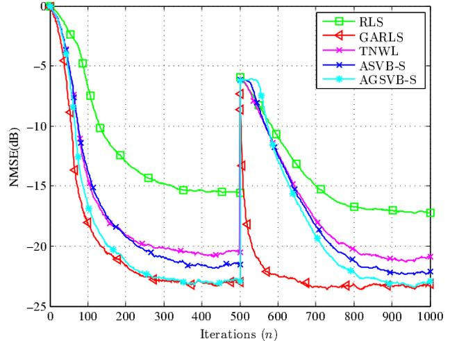
Fig. 1. NMSE curves under slow fading and a sudden channel change.
