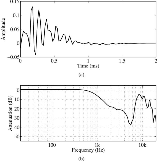
**Fig. 1:** Measured isolation properties of the supra-aural headphones, where (a) shows the windowed isolation impulse response and (b) shows the magnitude response. The sample rate is 44.1 kHz.
