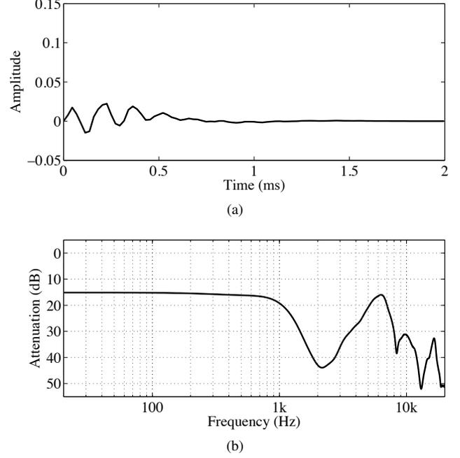
**Fig. 2:** Measured isolation properties of the in-ear headphones, where (a) shows the windowed isolation impulse response and (b) shows the magnitude response.
