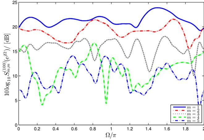
Fig. 4. PSDs  $S_{m,m}^{(100)}(e^{j\Omega})$  for SBR2 [1] demonstrating approximate spectral majorisation.
