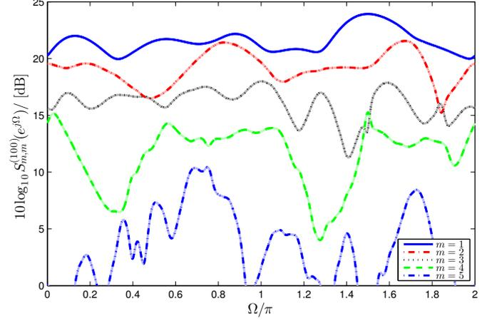
Fig. 7. PSDs  $S_{m,m}^{(100)}(e^{j\Omega})$  for C-MSME-SMD demonstrating approximate spectral majorisation.
