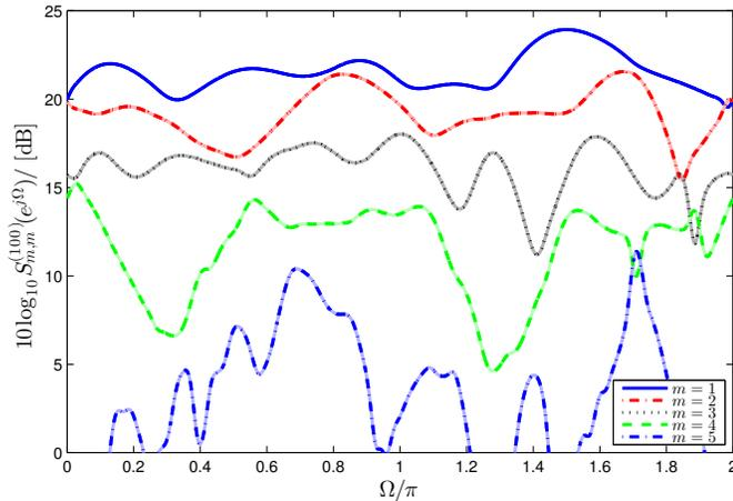
Fig. 6. PSDs  $S_{m,m}^{(100)}(e^{j\Omega})$  for MSME-SMD [10] demonstrating approximate spectral majorisation.
