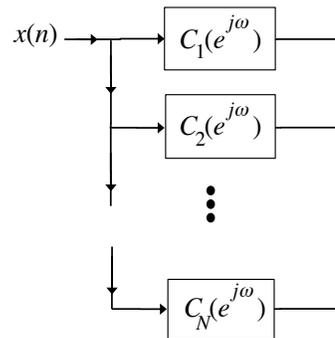
**Fig. 2.** The Ramanujan analysis filter bank.
