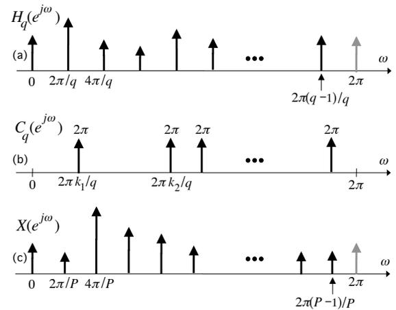
**Fig. 1.** (a) Frequency response of an arbitrary period- $q$  filter  $h_q(n)$ , (b) the frequency response of the ideal (infinite duration) Ramanujan filter  $c_q(n)$ , and (c) the Fourier transform of a typical period- $P$  signal.
