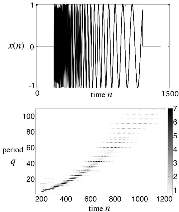
**Fig. 3.** A time-period plane plot obtained from the Ramanujan filter bank, for a inverse-chirp signal.
