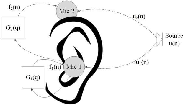
Fig. 1. Microphone arrangement [13]
