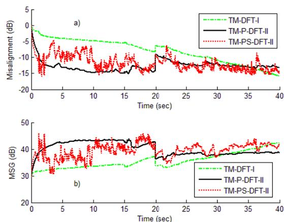
**Fig. 7.** (a) Misalignment and (b) MSG curves with music input, probe injection and feedback path variation at 20 seconds.
