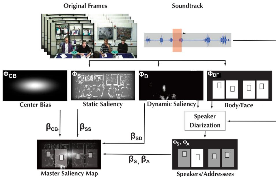
**Fig. 1.** Block diagram of our audiovisual saliency model. Center Bias, Static and Dynamic Saliency, Speakers and Addressees (Faces or Bodies) maps are weighted with the  $\beta^{Lasso}$  estimated weights, and merged into the audiovisual Master Saliency map.
