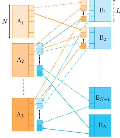
**Fig. 1:** Illustration of the distributed architecture. Nodes of group A (orange blocks) do parallel calculation w.r.t. the frequencies, while nodes of group B (blue blocks) do parallel calculation w.r.t. the pixels.
