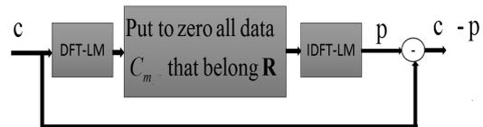
Fig. 3. Digital Frequency Domain Filtering scheme.
