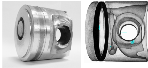
Fig. 1. Example of use for Inline-CT: Inspection of aluminum castings (e.g. combustion motor piston, left hand side) and colored visualization of the manufacturing defects (blue colored regions) within a reconstructed volume (right hand side).
