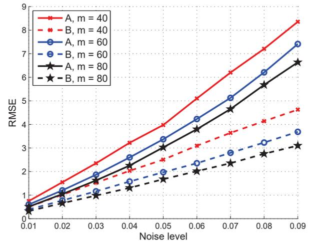
Figure 2: Estimation accuracy evolution for increasing noise levels and fixed number of sensors  $m \in \{40, 60, 80\}$  achieved by sensor networks whose positioning is given either by the random frame  $\mathbf{A}$  or by the closest  $s$ -tight frame  $\mathbf{B}$ .
