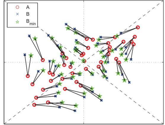
Figure 1: A two-dimensional sensor network with  $m = 40$  sensors positioned by a random frame  $\mathbf{A}$  and two tight frames  $\mathbf{B}$  (8) and  $\mathbf{B}_{\min}$  (16) computed from  $\mathbf{A}$ . The displacements of the sensors in the initial network, due to the tightness constraints, are depicted by arrows. The sensors are placed in an area of size  $1\text{km} \times 1\text{km}$ .
