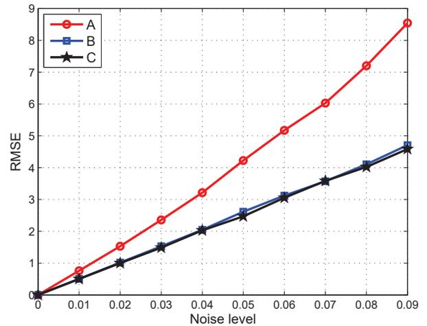
Figure 4: Estimation accuracy evolution for increasing noise levels and fixed number of sensors  $m = 40$  achieved by sensor networks whose positioning is given either by the random frame  $\mathbf{A}$  or by the closest  $s$ -tight and symmetric  $s$ -tight frames  $\mathbf{B}$  and  $\mathbf{C}$ , respectively.
