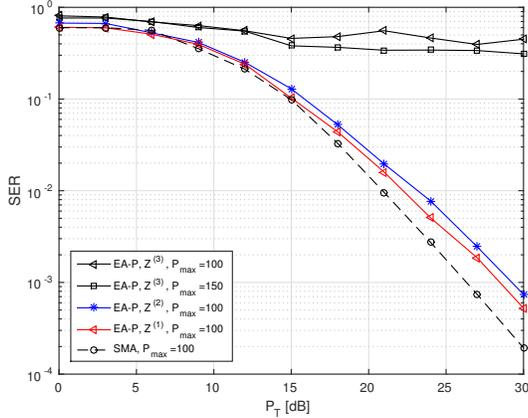
**Fig. 3:** SER performance comparison of the ESPAR transmitter and the standard multiple antenna transmitter employing Alamouti scheme with 16-QAM modulation.
