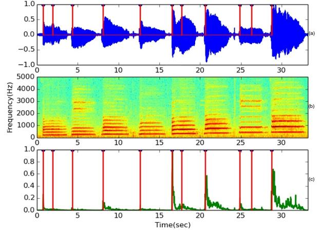
Fig. 2. (a) Time domain SARGAM note sequence and the overlaid detected note onset markers, (b) corresponding spectrogram, and (c) onset detection function and the overlaid detected onset markers (vertical red markers).
