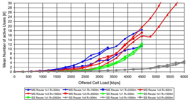
Fig. 7. Mean number of active MSS and SS users/sessions vs. cell load for a 3.5 MHz channel in 1x1 and 1x3 reuse for MSS, SS and varying cell size.
