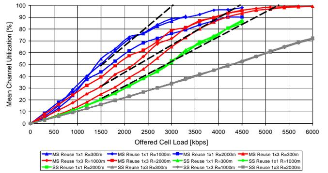
Fig. 8. Mean channel utilization vs. cell load for a 3.5 MHz channel in 1x1 and 1x3 reuse for MSS, SS and varying cell size.
