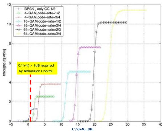
Fig. 2. Link level throughput vs.  $C/(I+N)$ , 3.5 MHz OFDM channel.
