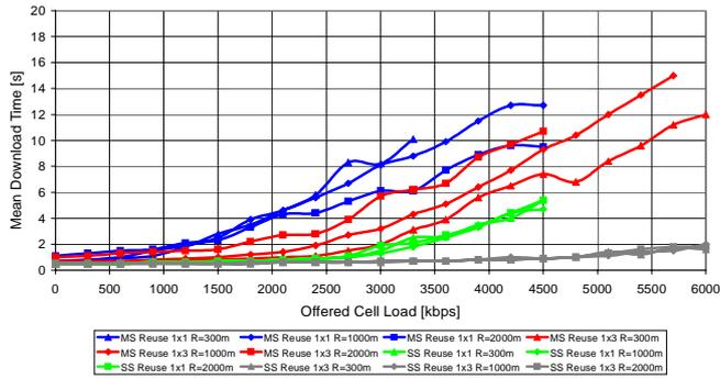
Fig. 6. FTP 300 kByte mean download time vs. cell load for a 3.5 MHz channel in 1x1 and 1x3 reuse for MSS, SS and varying cell size.
