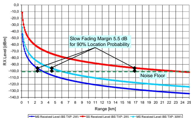
Fig. 3. Received signal level vs. range for MSS and SS.
