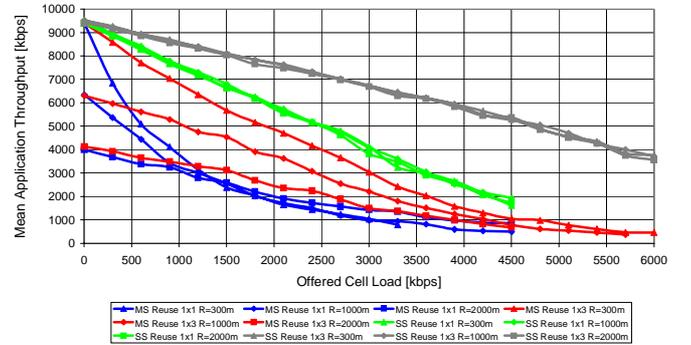
Fig. 5. FTP 300 kByte mean application throughput vs. cell load for a 3.5 MHz channel in 1x1 and 1x3 reuse for MSS, SS and varying cell size.
