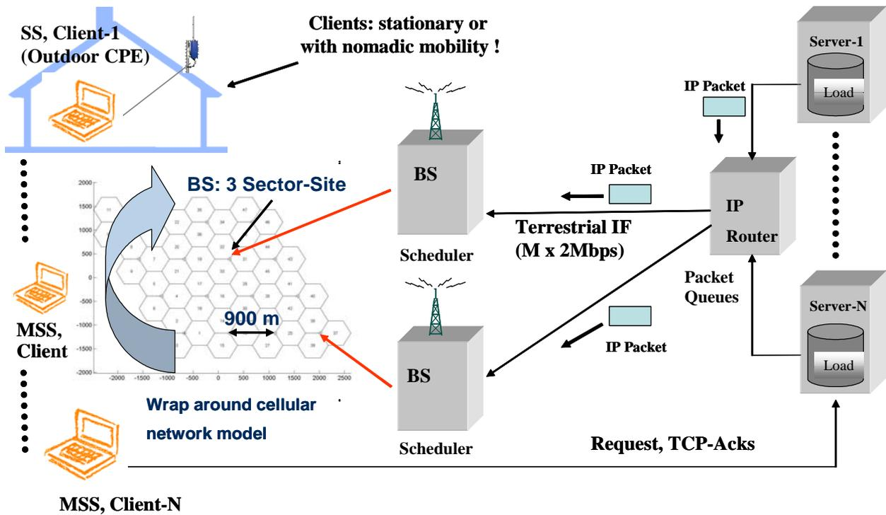
Fig. 1. IEEE802.16 (WiMax) OFDM System Level Simulation Model supporting both mobile subscribers (MSS) and fixed subscribers (SS).
