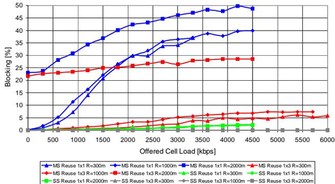
Fig. 10. MSS and SS packet call blocking vs. cell load for a 3.5 MHz channel in 1x1 and 1x3 reuse for varying cell size.
