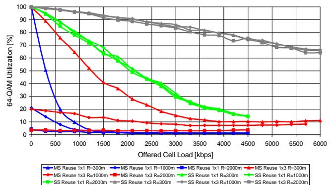
Fig. 9. QAM-64 utilization vs. cell load for a 3.5 MHz channel in 1x1 and 1x3 reuse for MSS, SS and varying cell size.
