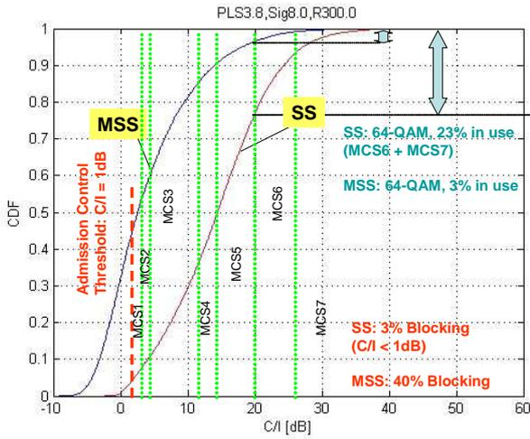
Fig. 4a. CDF of C/I and MCS utilization in 1x1 reuse at 100% system load.
