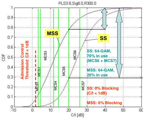
Fig. 4b. CDF of C/I and MCS utilization in 1x3 reuse at 100% system load.
