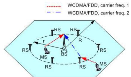
Figure 1. Enhanced uplink UTRA-FDD with fixed relay stations
