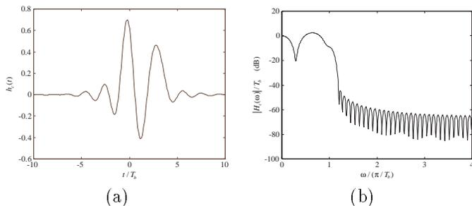
Figure 1: Received pulse shape (a) Time domain (b) Continuous frequency domain
