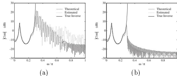
Figure 2: Identified inverse channel in discrete frequency domain (a)  $\mathbf{c}' = \mathbf{R}^{-1}\mathbf{d}$  (b)  $\mathbf{c}' = \mathbf{R}^+\mathbf{d}$
