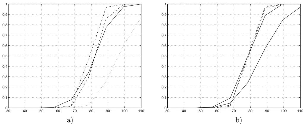
Figure 3: Results of the experiments of probability of detection ( $L= 15$  pixels). a) isotropic is shown dotted, censored isotropic dashed, integrator solid and gradient guided dashdotted. b) Integrator and gradient guided (solid and dashed resp.) for two target areas. The isolated curve in the figure corresponds to a  $8 \times 8$  pixels target. Both in a) and b) the magnitude in abscisae is the difference between the target mean intensity and the background mode.
