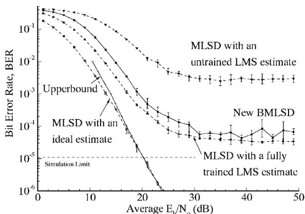
**Figure 3 BER Performance of BMLSD over a Fast Fading Three Path Channel with DQPSK Data**
