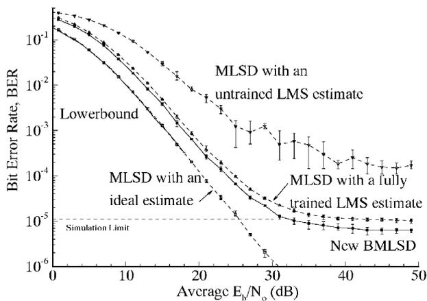
**Figure 2 BER Performance of BMLSD Over a Fast Fading Two Path Channel with DBPSK Data**
