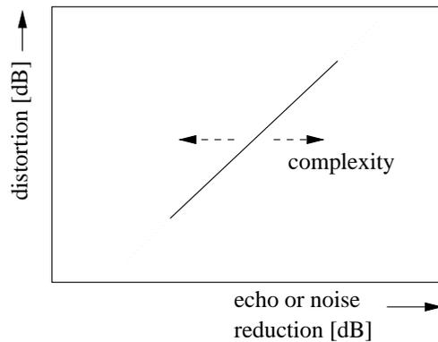
Figure 2: Qualitative plot of the near end speech distortion vs. the echo or noise reduction characteristics for combined systems.
