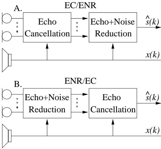
Figure 1: Processing configurations for combined systems: A) EC precedes ENR, B) ENR precedes EC.
