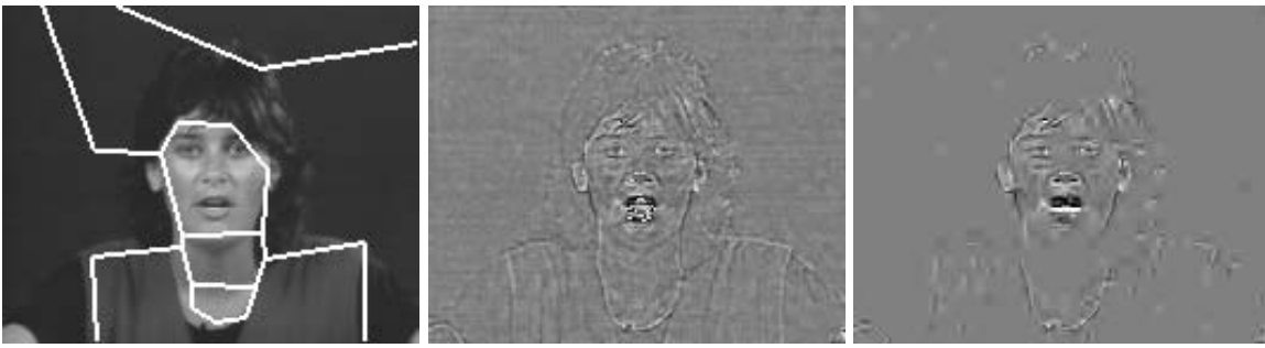
Figure 7: Images extracted from the sequences : the original image and its segmentation map, the corresponding prediction errors image and the vector quantized prediction errors image (differential images are centered and scaled 5 times).
