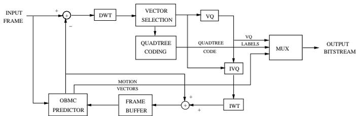
Figure 1: Adaptive subband VQ video codec
