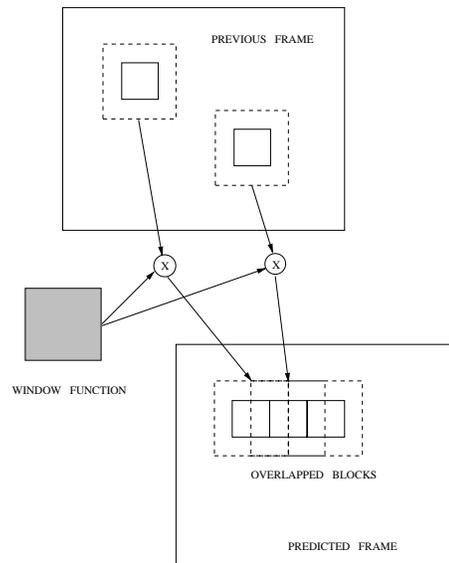
Figure 2: Overlapped block motion compensation
