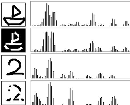
**Fig. 2 Vector representations formed by the unity resolution PAP-method (N=1) for several patterns.**
