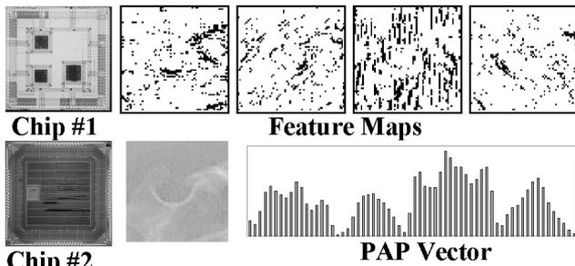
**Fig. 8 Photomicrographs of dedicated VLSI chips and feature maps and a vector for a Sella (a pituitary gland) pattern generated by chip #2 at 25 MHz.**
