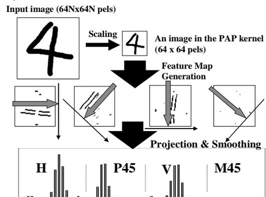
Fig. 1 Characteristic vector formation by Multi Resolution Principal Axis Projection (MRPAP).
