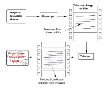
Figure 1: A block diagram of the system causing moiré degradation.
