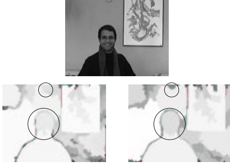
Figure 4: Comparison of the effect of edge detection on the segmentation. Segmentation of the image Sergi. Level of segmentation: \sigma_n = 25 pixels (left: not using edges, right: using edges).
