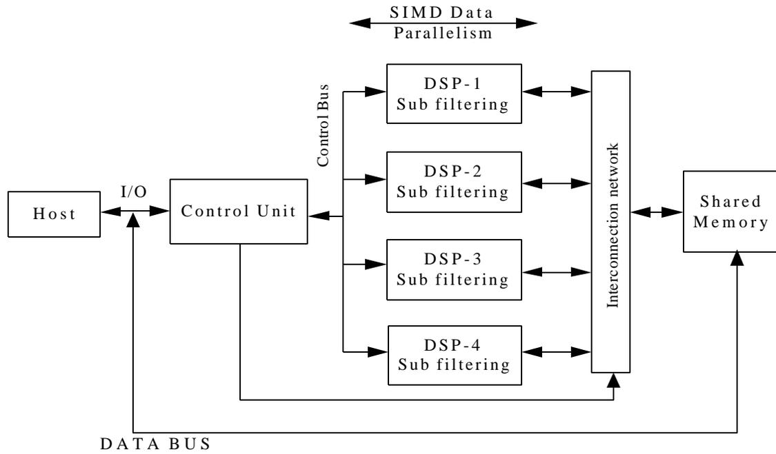
**Figure 2. Multiple DSPs System Architecture for 2-D Parallel Image Filtering.**
