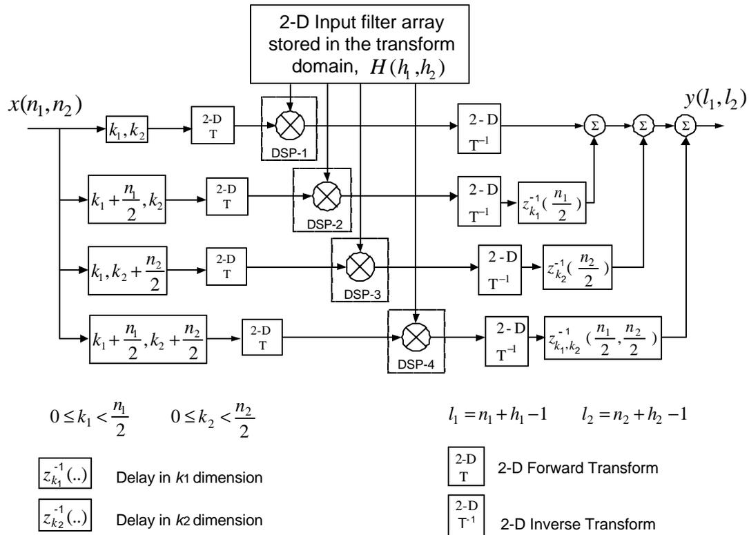
Figure 1. 2-D Parallel Block-Filtering Using Overlap-Add for Image Processing
