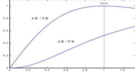
Figure 2: Normalized non-linear model characteristics.
