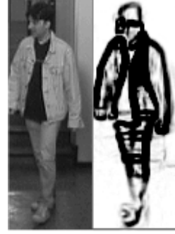
Figure 1: Example of the variance map generated by the change detector. Darker regions correspond to a larger variance.
