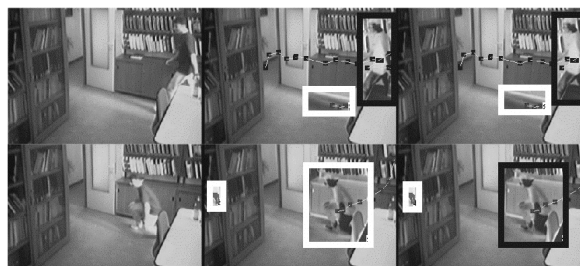
Figure 5: Example of application. From left to right: original frame, output of the attention focusing block, output of the final classification block. In the top sequence the intruder is correctly detected already at the second stage of the algorithm. In bottom sequence a correct classification is only achieved with the third phase.
