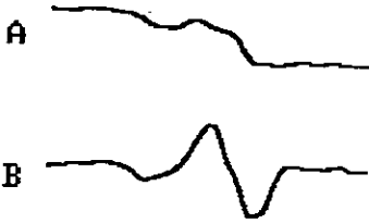
Fig. 4. Example of the brightness profile of a scanline (A) and the derivative function (B).
