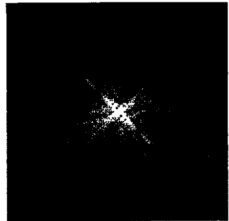
Fig. 2b — Equalized magnitude spectrum of 1b.
