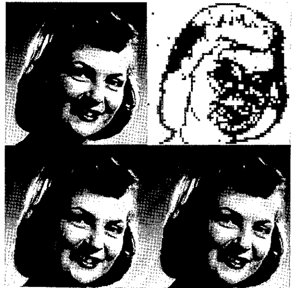
Fig. 3. The results of Modified BTC algorithm. Starting from the top left clock-wise: a. the original 8bit/pel, b. block classification, c. reconstructed image (0.6 bit/pel), d. reconstructed image after selective interpolation post-filter (0.6 bit/pel).
