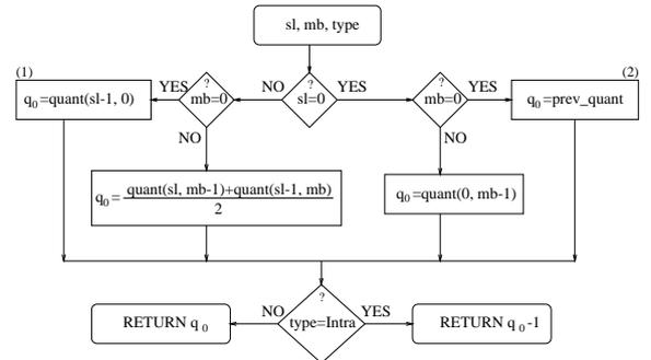
Figure 3: Algorithm scheme for the calculation of the quantization factor  $q_0$ .
