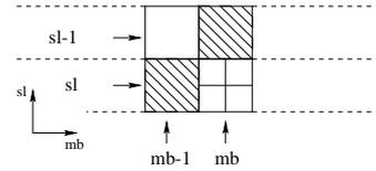
Figure 2: Scheme of the  $\Phi$  set for the macroblock  $mb$  of the slice  $sl$ . There are also shown the four blocks of the current macroblock.
