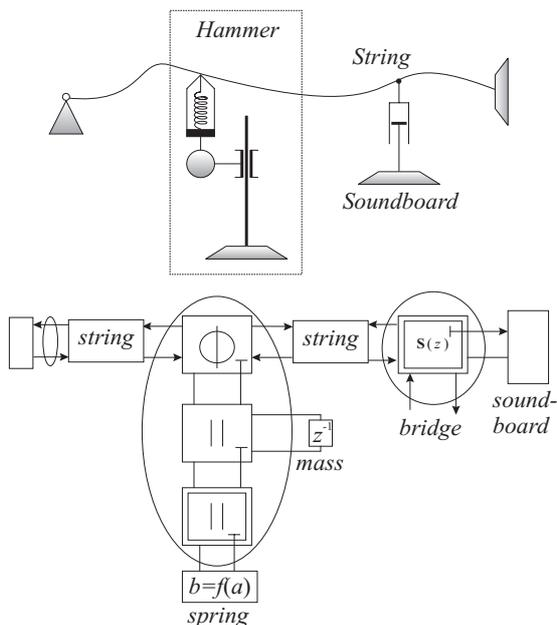
Figure 3: Physical model of a piano and its WD implementation.
