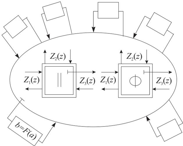
Figure 1: General synthesis scheme of a WD structure: blocks are either filters or instantaneous nonlinearities; adaptors are dynamic.
