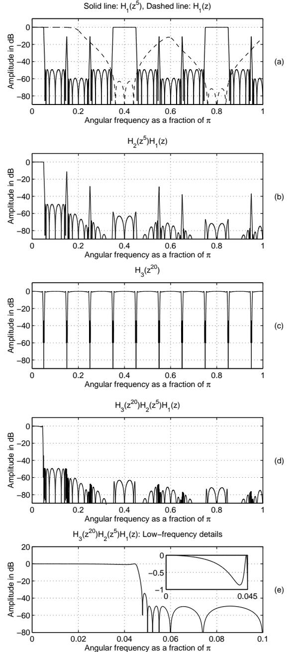
Figure 6: Design of a 20-to-1 decimator using two  $N$ th-band recursive filters and a corrector filter at the output sampling rate.
