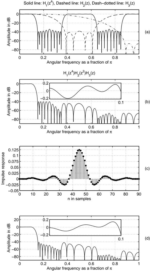
Figure 3: Responses for three-stage filters of Example 1. (a) Amplitude responses for the subfilters. (b) and (c) Amplitude and impulse responses for the overall minimax  $N$ th-band FIR filter. (d) Amplitude response for the least squared filter design.
