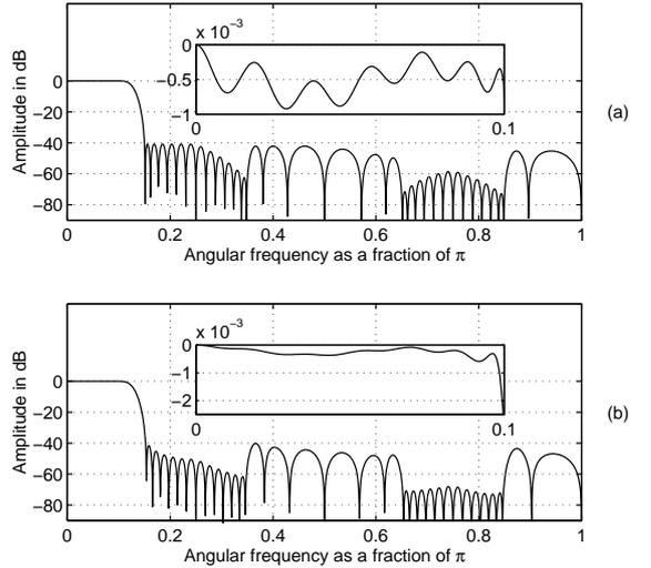
Figure 4: Responses for three-stage filters of Example 2. (a) Common amplitude response for  $T(z)$  and  $R(z)$  designed in the minimax sense. (b) Common amplitude response for  $T(z)$  and  $R(z)$  designed in the least-mean-square sense.
