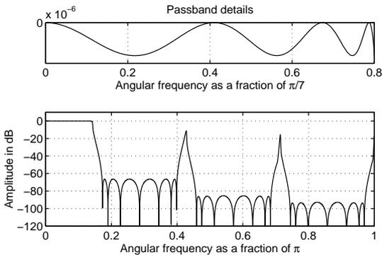
Figure 5: Amplitude response for a seventh-band IIR filter.
