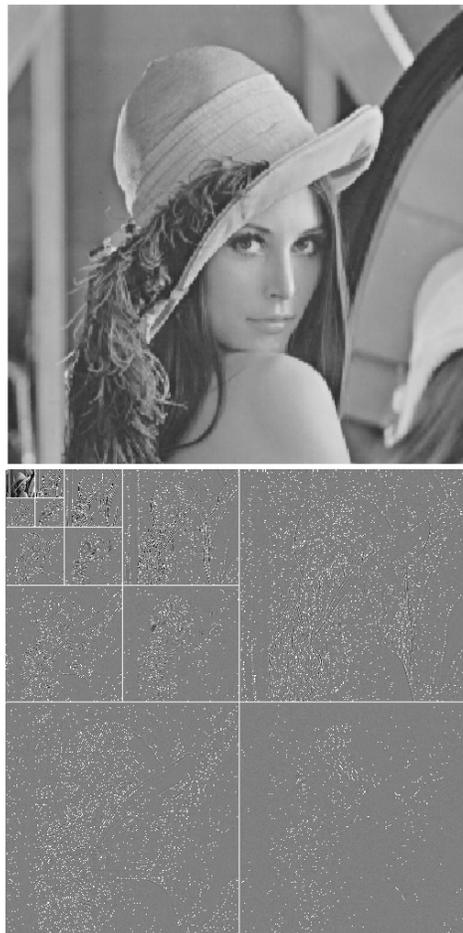
Figure 2: Original test image Lenna (top), and the same image decomposed into 13 bands by a discrete wavelet transform (bottom).
