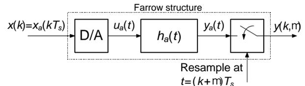
Fig. 1. The hybrid analog/digital model for the interpolation filter.
