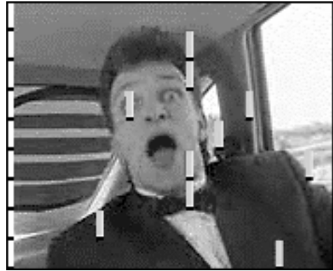
Figure 2: Resynchronization markers for a QCIF frame. The GOB headers are shown in white along the left edge of the image while the Slice Structure Mode headers are dispersed throughout the frame at 512 bit intervals in the bitstream.
