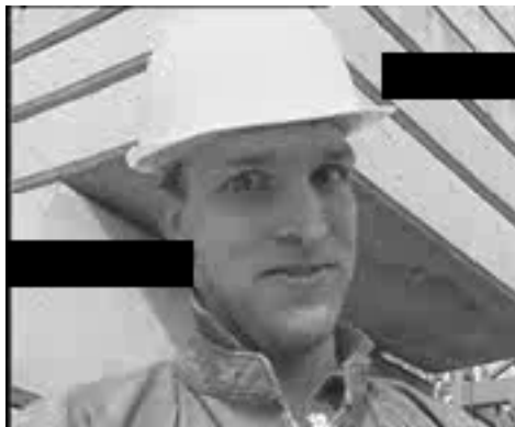
Figure 5: Missing macro block location of 14th frame of "Foreman" sequence (inter frame)
