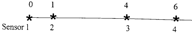
Figure 3 : Non redundant array of four sensors. The stars represent the sensors. The numbers represent the sensor positions.
