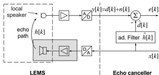
Figure 1: Nonlinearities in the electro-acoustic echo path (shaded area)
