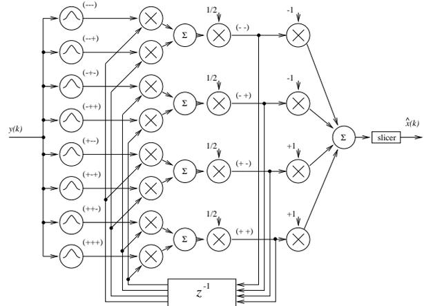
**Figure 4:** Recurrent MAPSD for  $N = 3$ . (The notation  $(+++)$  on the layer of basis functions indicates the scalar centre which has been used e.g.  $(+++)$  implies the centre  $[+1, +1, +1]\mathbf{h}$ . The notation  $(+-)$  indicates the values of the channel inputs upon the densities are conditioned e.g.  $(+-)$  indicates densities conditioned on  $x(k) = +1$  and  $x(k-1) = -1$ .)
