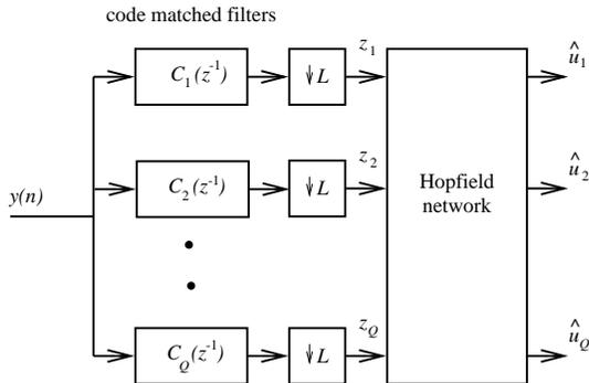
Figure 9: Hopfield neural network detector for synchronous CDMA
