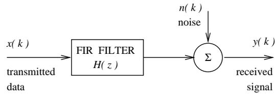
Figure 1: Digital communications channel
