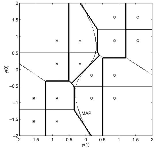
**Figure 2:** Observation space for  $H(z) = 0.35 + 0.87z^{-1} + 0.35z^{-2}$  showing MAP decision boundary for  $d = 1$  and MLSE boundaries.
