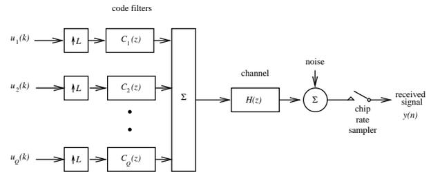
Figure 7: Discrete-time model of CDMA downlink.
