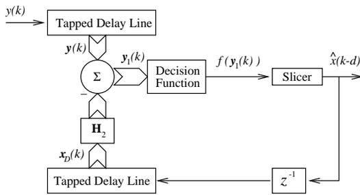
Figure 6: Decision feedback MAPSD with linear feedback network  $H_2$
