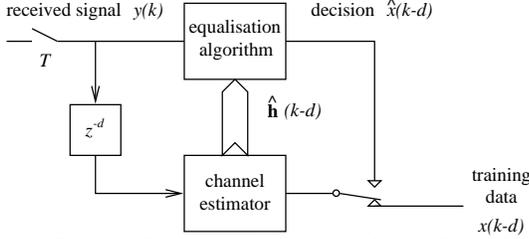
**Figure 3:** Generic adaptive equaliser for mobile radio applications
