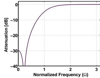
Figure 6: Transfer function  $H(z)$  of the second order highpass
