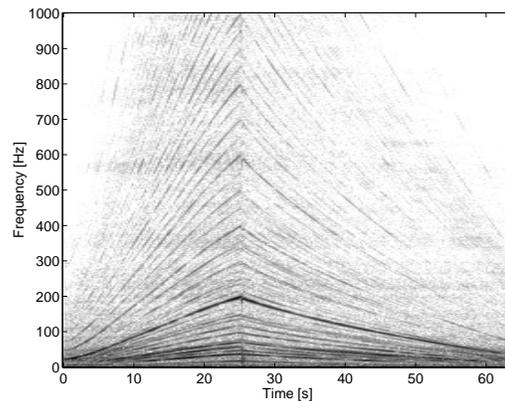
Figure 1: Spectrogram of a typical engine noise
