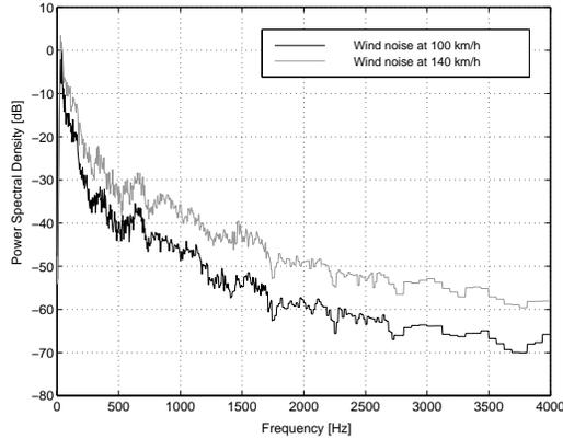
Figure 3: Wind noise at two different speeds
