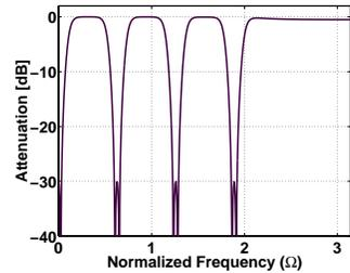
Figure 8: Transfer function of the modified notch filter  $G(z)$
