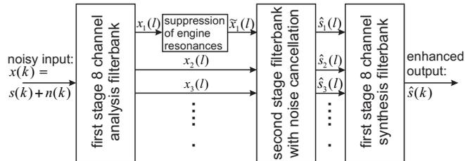
Figure 9: Structure of the noise cancellation algorithm composition is followed by a second, which is required by the noise reduction algorithm to remove the other noise components. We obtained satisfying results with this filtering in time, especially without speech distortions.
