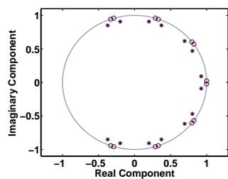
Figure 7: Poles (\*) and zeros (o) of the modified notch filter  $G(z)$
