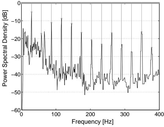
Figure 2: PSD of engine noise at 3485 rpm
