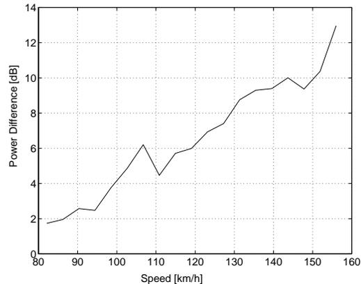
Figure 10: Power of wind and tyre noise dependent on the car speed referred to the power at 80 km/h
