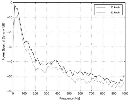
Figure 4: Tyre noise at different speeds depicted in Fig. 4 for two different speeds. Even though
