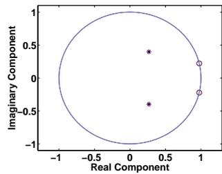
Figure 5: Poles (\*) and zeros (o) of the second order highpass  $H(z)$
