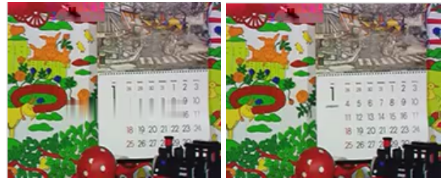
Figure 2: Left and right pictures reconstructed respectively by JVT and our proposed algorithms in case of a corrupted Intra frame.
