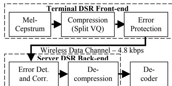
Figure 1: The Aurora standard for a DSR architecture.
