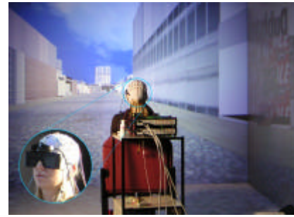
Figure 2: Walking in a virtual street by "thought". This experiment was performed by the Graz BCI team in June 2004 in the CAVE (Computer Animated Virtual Environment) of the University College of London (UCL).
