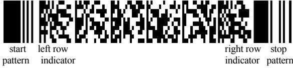
Figure 3. A PDF417 bar code including 10 rows and 4 columns.
