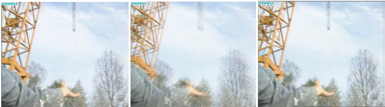
Figure 4. "Foreman" Sequence. Left: An original image, Center: An image interpolated by using a fading from the two more near available images. Right: An image interpolated by using a motion compensated strategy.
