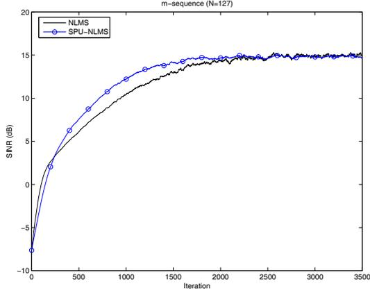
Figure 4: NLMS vs SPU-NLMS in blind MUD ( $N = 127$ ).
