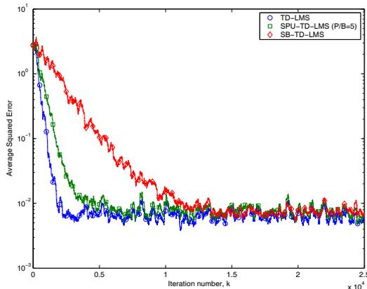
Figure 2: Convergence comparison for TD-LMS and SPU-TD-LMS in acoustic echo cancellation example.
