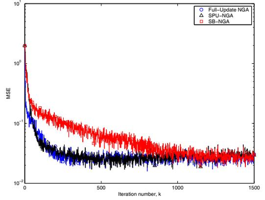
Figure 3: Converge comparison for blind channel equalization algorithms NGA and SPU-NGA.
