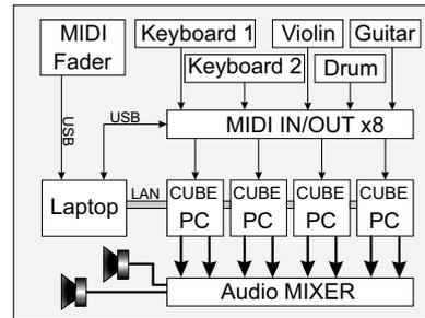
Figure 4: Block diagram of the live performance system.
