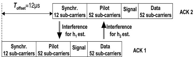
Figure 2: Interference to channel estimation over ACK bursts.
