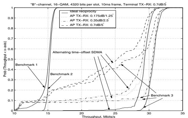
Figure 6: Throughput performance for two users and three-antenna AP in the "D"-channel 5.2 GHz environment.
