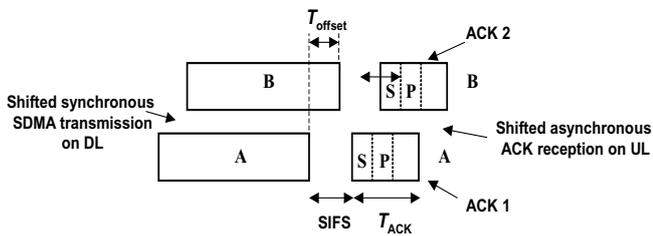
Figure 1: Time-offset SDMA slot for two users.
