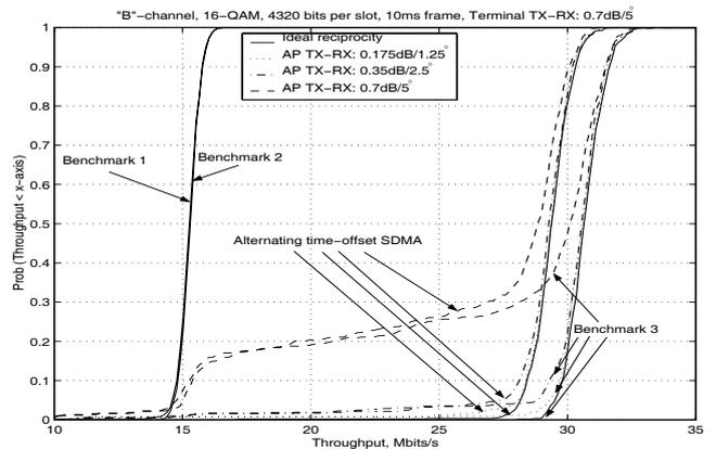
Figure 5: Throughput performance for two users and three-antenna AP in the "B"-channel 2.4 GHz environment.
