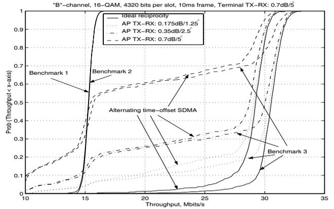
Figure 4: Throughput performance for two users and two-antenna AP in the "B"-channel 2.4 GHz environment.
