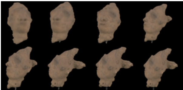
Fig 4: Streaming scenario: (First row) a) initialization with coarse model at r = 6 , b) after rotation with \Delta\theta = 30^\circ , c) r = 7 , d) after rotation with \Delta\theta = 30^\circ ; (second row) e) r = 8 , f) after rotation with \Delta\theta = 30^\circ , g) r = 9 , h) after applying all available geometric precision.
