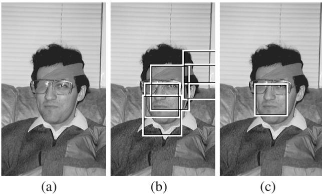
Fig. 9. Results of face segmentation (b) and verification (c) from original face image (a) whose right eye is occluded.
