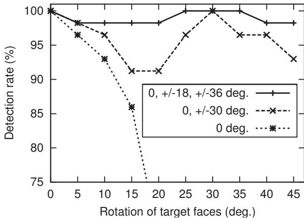
Fig. 4. Detection rate from rotated target images with different combinations of tilted template vectors.
