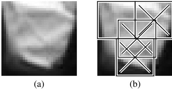
Fig. 8. An example of false positives in face segmentation (a); this was rejected in verification since only a right eye passed facial-parts validation (b).
