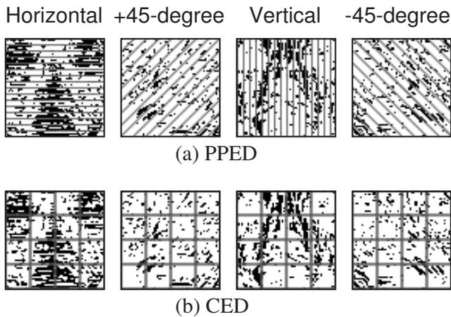
Fig. 2. Partitions of feature maps for vector generation based on projected principal-edge distribution (PPED) (a) and cell edge distribution (CED) (b).
