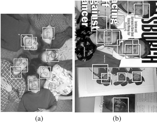
Fig. 5. Results of rotation-invariant face segmentation using image in Ref. [13]. Face verification was not conducted in this experiment.
