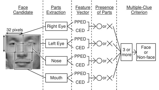
Fig. 3. Face verification using finer edge information of eyes, nose and mouth.
