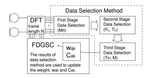
Figure 3: The procedure of the three phase data selection method.
