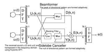
Figure 2: Target sound extraction using the FDGSC.
