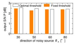
Figure 11: Output S/N when using the optimal threshold and the fixed threshold(the received sound S/N was set to -3[dB]).
