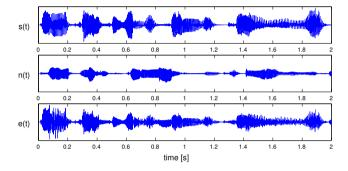
Figure 9: Waveform: s(t) is the target sound, n(t) is the noisy sound and e(t) is the extracted sound.
