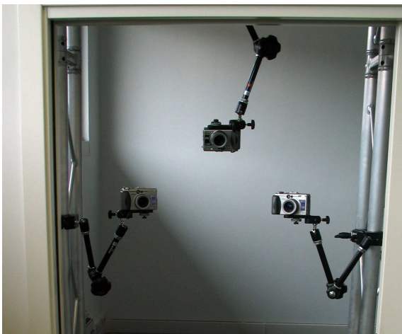
Figure 2: The acquisition system. Three cameras placed around a gate.
